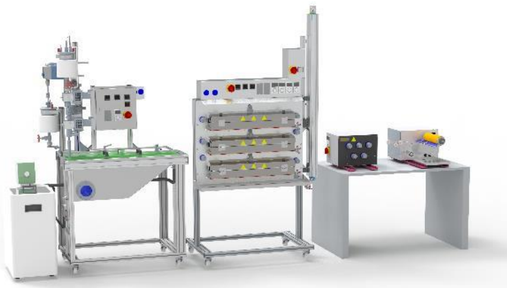
Lab scale line for wet spinning
